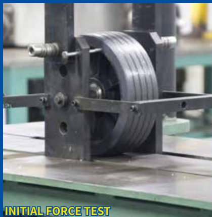
Extra Heavy Dynamic Rolling Tester Max load Capacity up to 20t. Max speed up to 16 km/h
